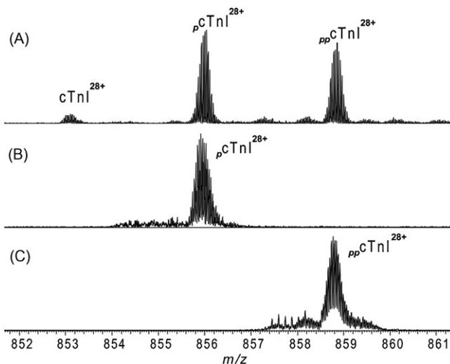
**Fig. 3.** Isolation of a single charge state ( $M^{28+}$ ) of *Rhesus* monkey cTnI phosphorylated ions. A, a mixture of un-, mono- and bis-phosphorylated cTnI; B, mono-phosphorylated cTnI; C, bis-phosphorylated cTnI.
